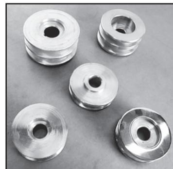
The diameter of the alternator pulley is very important. In order to insure a strong output from the alternator at idle and low rpms, it is important that the alternator pulley be at or close to (2.5") in diameter.
