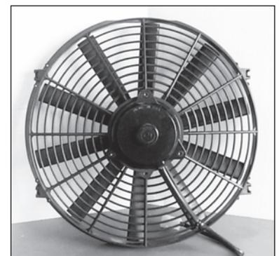
Adjustable metal brackets that mount the fan assembly to the outside framework of the radiator is the best choice for mounting the fan. Nylon ties that use the radiator core for support will damage the radiator core.
