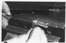
It is recommended that an additional 5" of wire extend beyond the casing so that it may be trimmed to exact length once the assembly has been installed in the vehicle.
